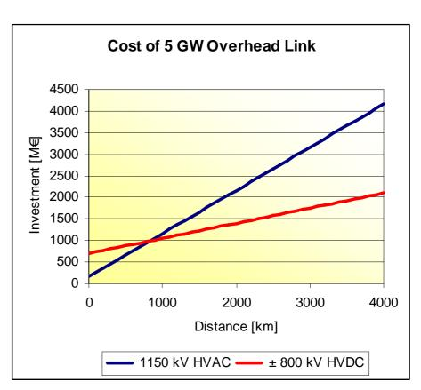
HVDC High Voltage Direct Current, HVAC High Voltage Alternating Current
